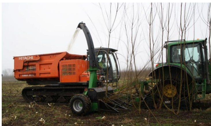
Figure 4.3: View of the tractor-pulled whole stem harvester (on the left) and the self-propelled cut-and-chip harvester with the trailer-tractor combination (on the right) operating at the same short rotation woody crop poplar plantation.
