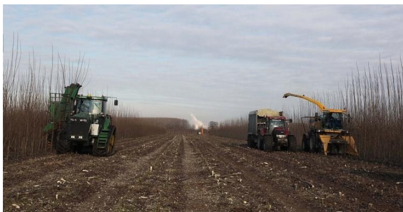
Figure 4.3: View of the tractor-pulled whole stem harvester (on the left) and the self-propelled cut-and-chip harvester with the trailer-tractor combination (on the right) operating at the same short rotation woody crop poplar plantation.
