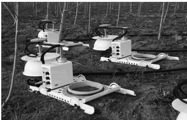
Figure 7.1: The LI-8100 soil chambers in operation at the field site (photo M.S. Verlinden).
